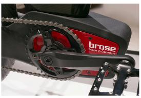
The motor unit used in the Brose design study.
